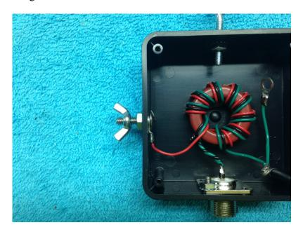
Install the other 6-32 Phillips flat head screw through the bottom right hole of the SO-239 connector, place the green wire with the #6 ring lug on the screw and secure with a 6-32 K-lock nut. Tighten both screws on the SO-239 connector until the heads are flush on the outside of the box (be careful not to distort the plastic—you can use too much torque).
