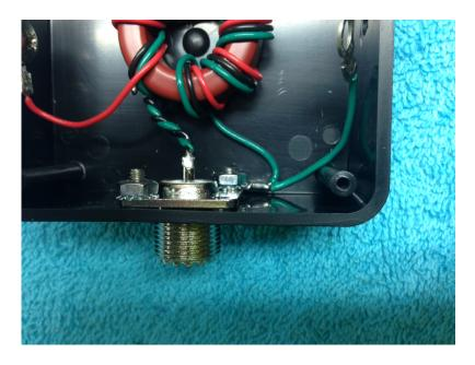
Finally, route the short green wire to the right and install the 10-24 Phillips truss head bolt through the ring lug and the hole in the box. Secure it with a 10-24 K-lock nut and tighten. Install the wing nut on the bolt.
