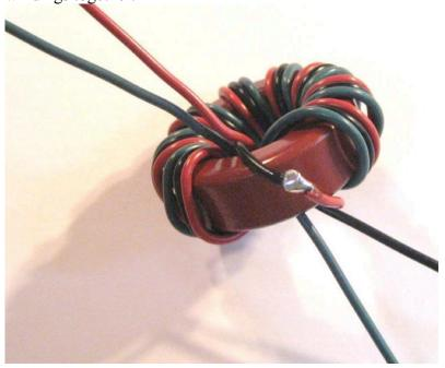
A few more steps and we'll have the transformer configured and ready to install in the box. Refer to the photo of the finished transformer for the next steps. (Note that the photo shows no ring lug at the end of the short green wire. This kit has a #10 lug at the end. Just follow my instructions You can also refer to the other photos.)
