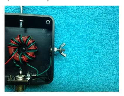
Secure the toroid to the bottom of the box using a dab or RTV silicone, Gorilla glue (what I use), or any other waterproof cement.
