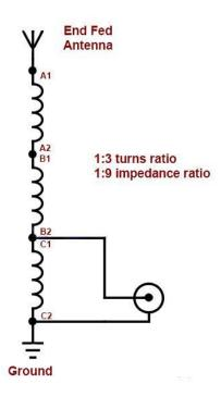
It is designed to match the high impedance of a non-resonant end fed antenna into a range where most antenna tuners and some internal tuners can produce good performance. As designed, the matchbox can handle up to 150 watts PEP.
